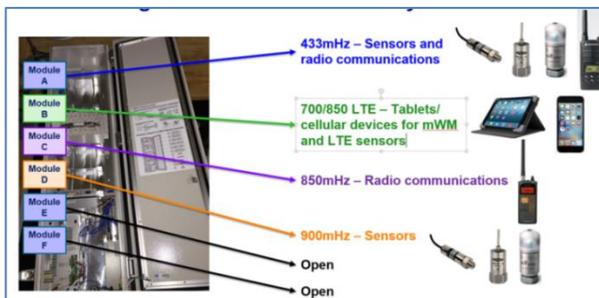
Figure 1: Modular DAS platform configured for power plant applications
