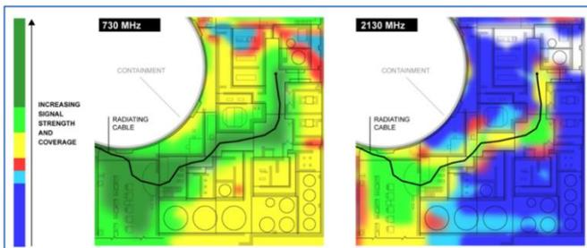
Figure 2: Signal coverage comparison of 730 MHz vs. 2,130 MHz frequencies inside a nuclear facility
